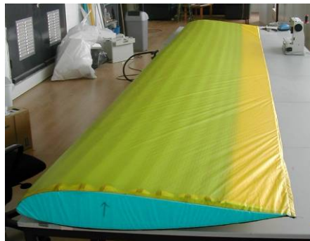
Figure 13. The complete 4 m 2 Tensairity kite after inflation.
