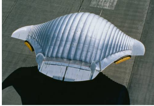
Figure 1. The manned inflated aircraft Stingray of ‘prospective concepts’.
