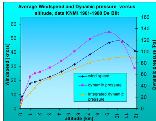
**Figure 1: Wind speed and dynamic pressure vs. altitude [3]**
