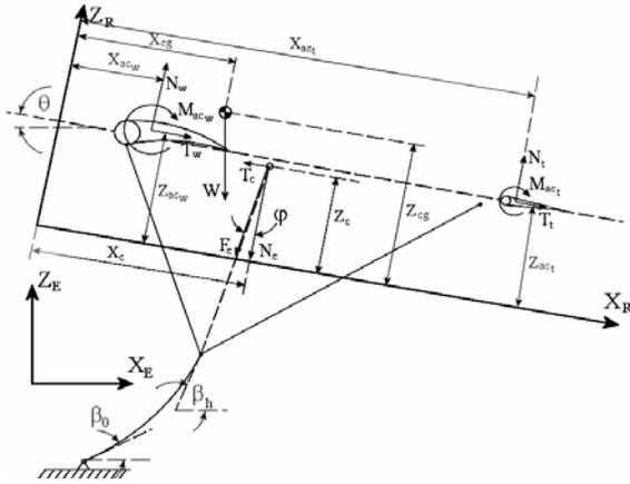
Figure 1: The forces on the kite in flight.
