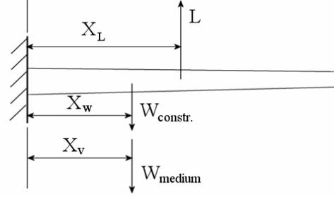
**Figure 6: The loads on the main spar**
