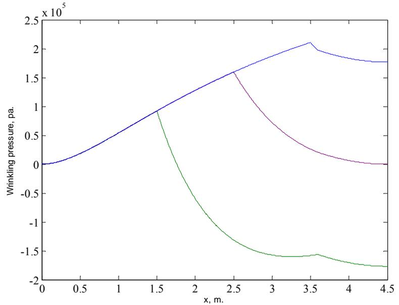
**Figure 11. Minimum internal pressures as a function of  $x$  for three different positions of the bridle line.  $b_2 = 1\text{m}$  in blue,  $b_2 = 2\text{m}$  in purple and  $b_2 = 3\text{m}$  in green.**
