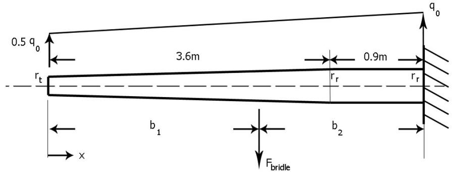
**Figure 10. The simplified loading of the kite wing.**
