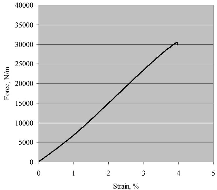
**Figure 7. Test result of the bonded laminate.**
