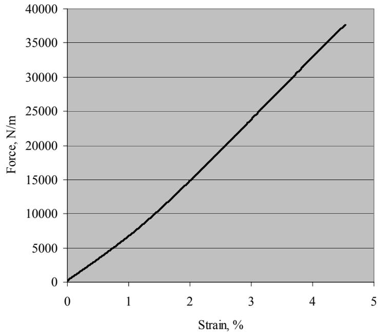
**Figure 6. Test result of the unbonded laminate.**
