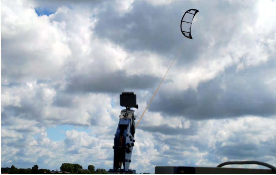
Fig. 2.1 A remote-controlled 25m 2 Leading Edge Inflatable (LEI) tube kite flying crosswind while pulling a 4mm cable with a force of 3kN from the ground station swivel, generating a traction power of 15kW [8]
