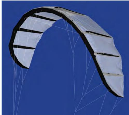
resolution Finite Element approaches such as depicted in Fig. 17.1 are too detailed for most purposes and correspondingly too expensive in terms of CPU time. Furthermore, fast and accurate aerodynamic load models that match the level of detail of such an FE model do not exist at present.
