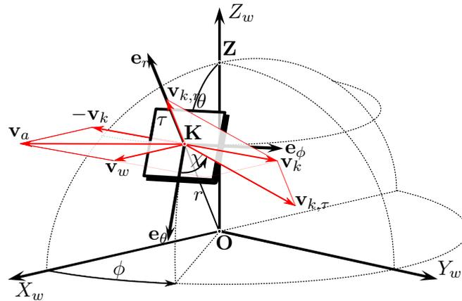
**Figure 2.** Definition of the apparent wind velocity  $\mathbf{v}_a = \mathbf{v}_w - \mathbf{v}_k$ . Decomposition of the kite velocity  $\mathbf{v}_k$  into radial and tangential components  $\mathbf{v}_{k,r}$  and  $\mathbf{v}_{k,\tau}$ , respectively. The course angle  $\chi$  is measured in the tangential plane  $\tau$ , the spherical coordinates  $(r, \theta, \phi)$  are defined with respect to the wind reference frame  $X_w, Y_w, Z_w$  [6].
