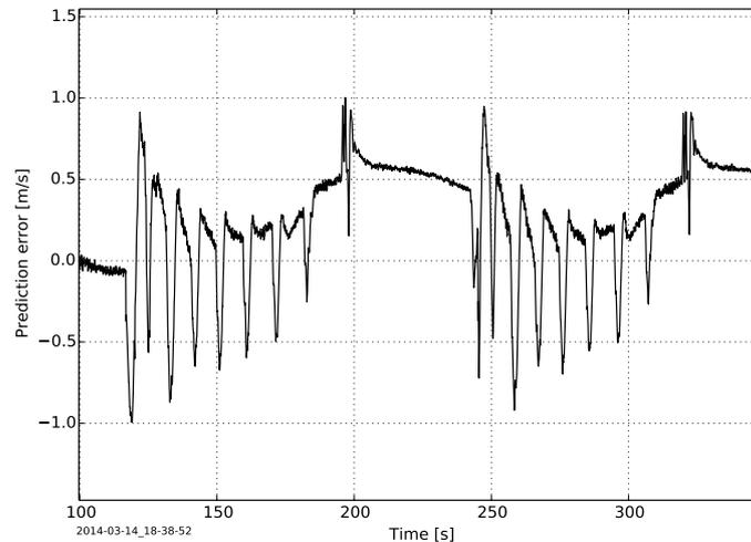
**Figure 3.** Prediction error of the reel-out speed during two power cycles with feedback control only. The measured force was used as set-force, and the difference between the measured and the predicted reel-out speed is shown. An error of 1 m/s is equivalent to about 7 % of the full range of the reel-out speed, that was used.
