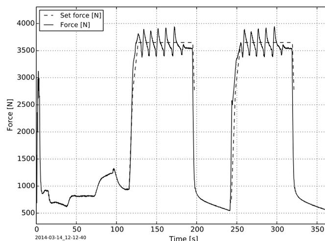
**Figure 4.** Set force and actual force of two power cycles with feedback control only. Where no set force is shown the controller is operating in constant speed mode. The set force has to be chosen such that the maximal design force of 4000 N is not exceeded.
