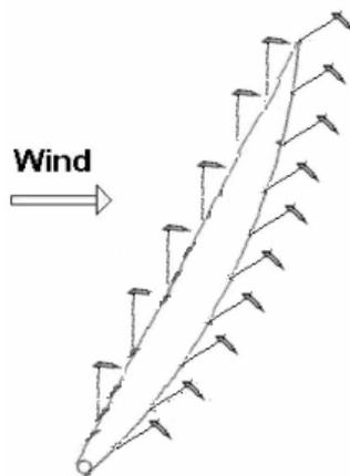
Figure 4: Laddermill with wings on ropes for cross wind power [after 1]
