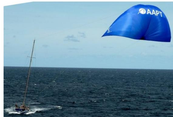
**Figure 12: Cloth kite replacing sails of a sailing boat [7]**
