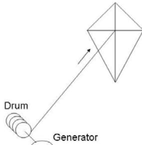
**Figure 2: Simple illustration of the Laddermill principle**
