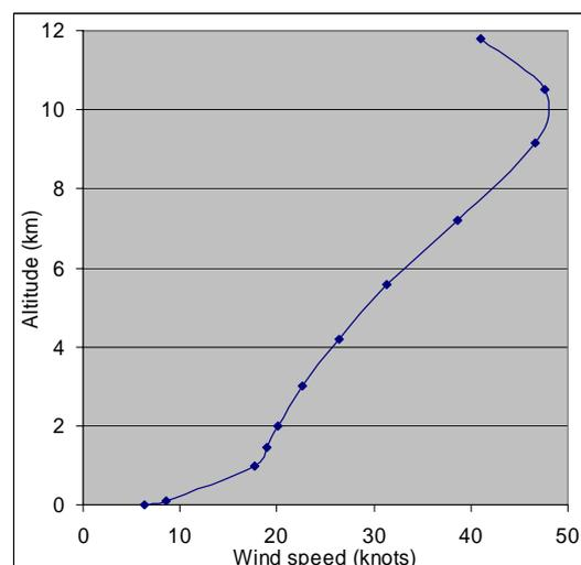
Figure 1: Average wind over the Netherlands versus the altitude [1]
