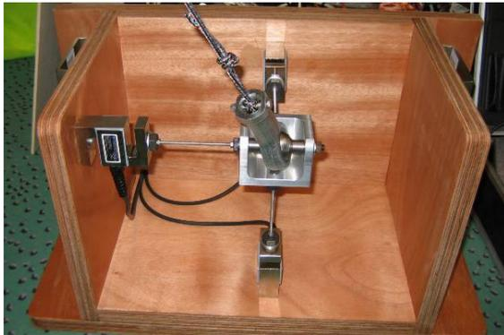
**Figure 26: Kite tension and direction sensor**
