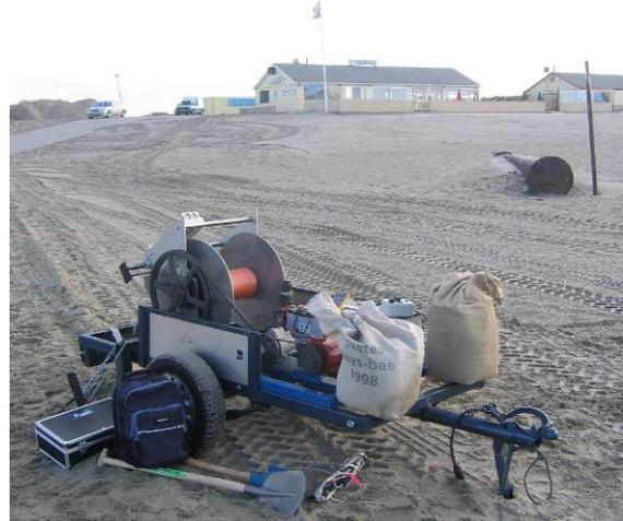
**Figure 20: 2 kW groundstation.**
