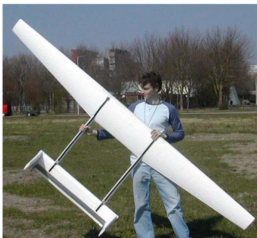
**Figure 4: A prototype for the laddermill wing**
