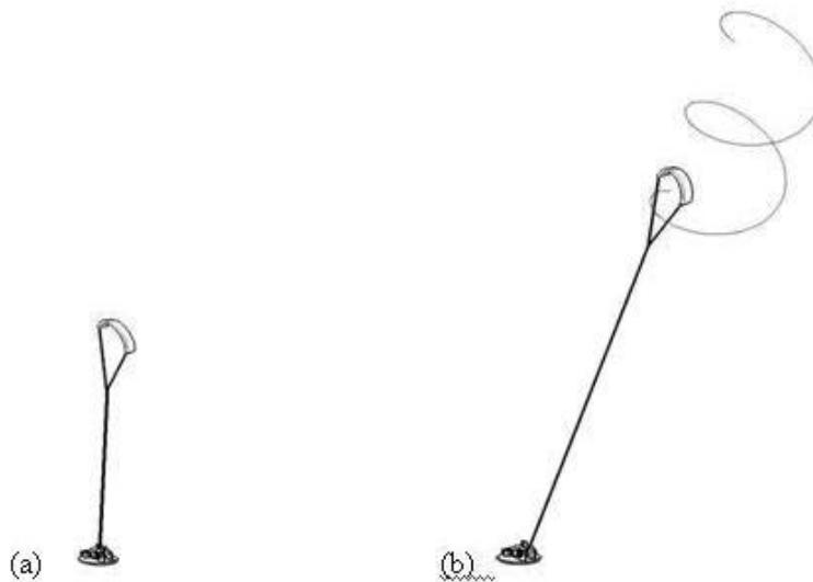
Figure 3. Laddermill concept. Panel (a) shows the laddermill in the downstroke phase, the kite is kept stationary with minimum angle of attack to minimize the line tension during retraction. The right panel shows the laddermill in the upstroke, the kite is moved through the flight envelope to generate a higher apparent wind speed and in combination with a high angle of attack generates a high line tension. During this phase the Laddermill generates electricity
