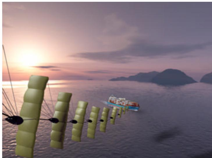
Fig.1 Results of a student design exercise, showing a series of smart kites each fitting in a standard container. The study included the deployment and retrieval of the kit
