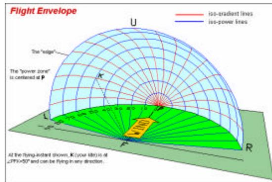
Figure 2. The flight envelope (Seattle Airgear)
