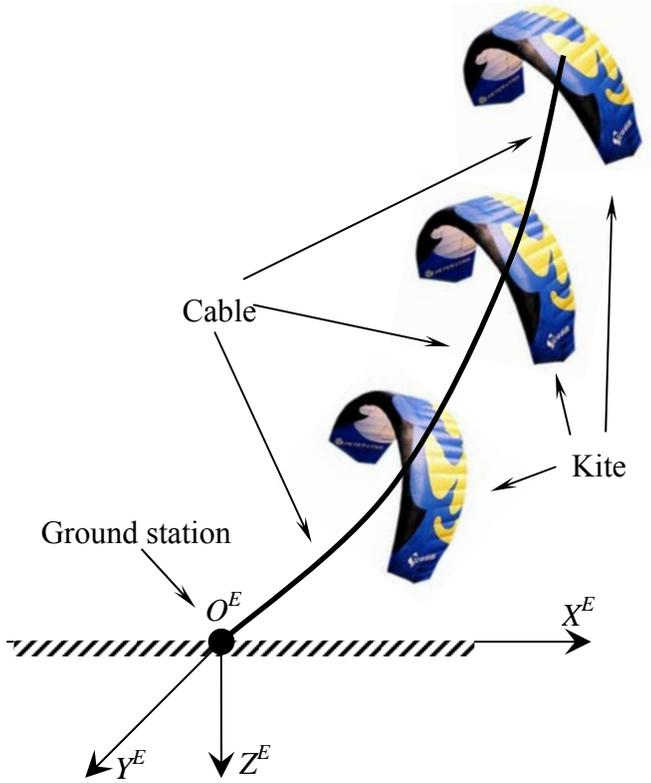
Fig. 1. The general structure of the Laddermill and Earth-fixed reference frame
