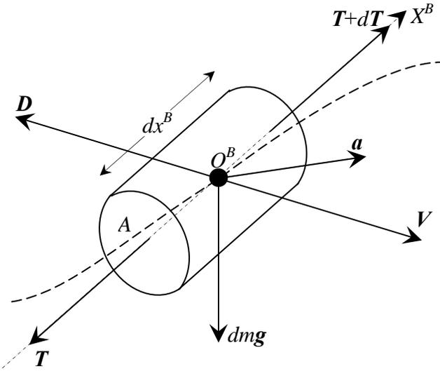
Fig. 4. Forces acting on a cable
