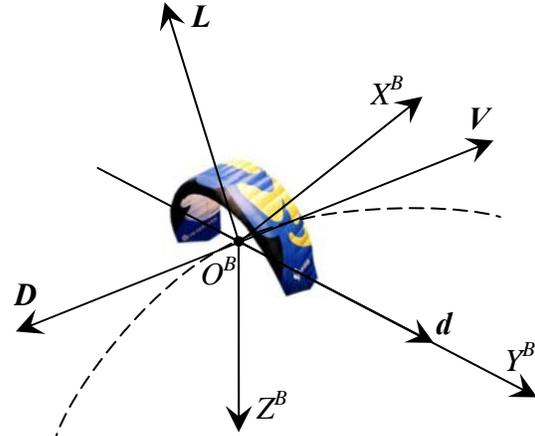
Fig. 2. Aerodynamic forces and kite's attitude in body-fixed reference frame
