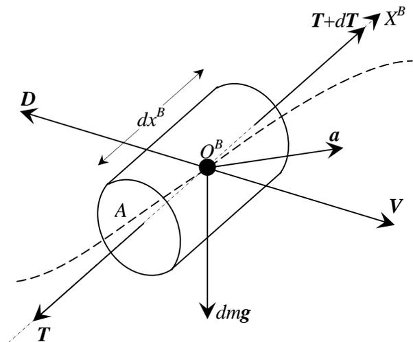
Fig. 6. Forces acting on a cable element
